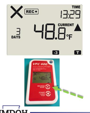
An X, in the upper left corner means the temperature has been <u>out</u> <u>of range</u>.
