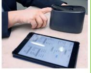
team brought their veggie a newly developed device that gives a score for how many fruits and vegetables a person eats over time. The Veggie Meter uses an LED light and complex physics to detect nutrients in our skin called carotenoids. These nutrients build up in our bodies when we a variety of fruits and vegetables. You put your finger in the device for 25 seconds to get a reading. The Veggie Meter is completely harmless. Why are carotenoids important?
